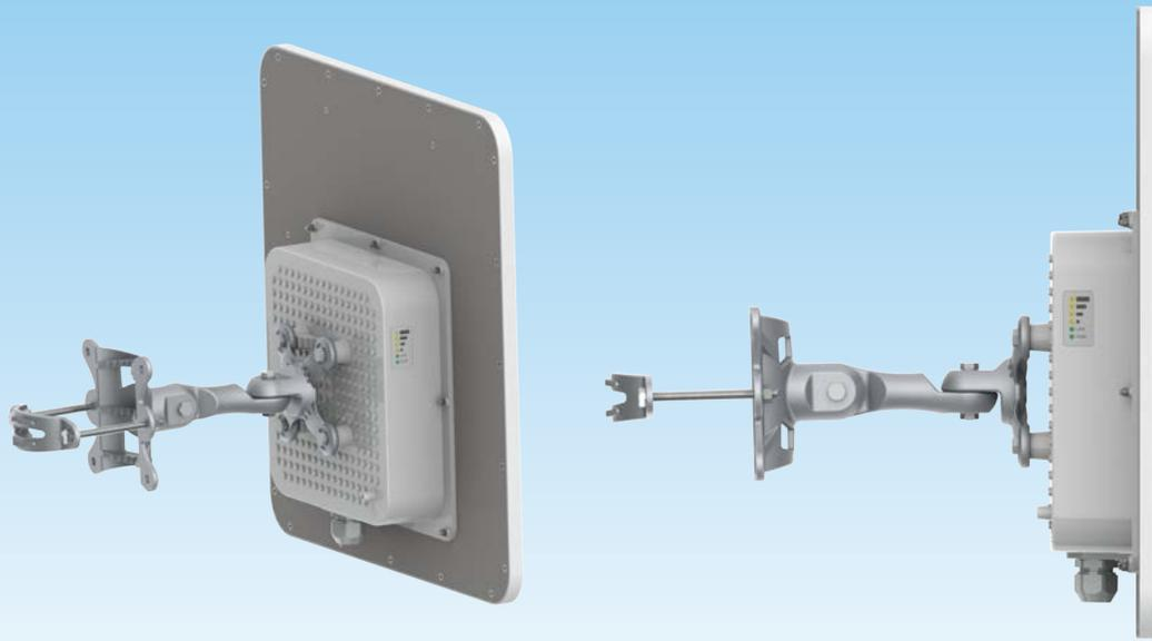
The APC Mach 5 presents a 5 GHz point-to-point product with superior performance building long distance links. This product is equipped with an extreme output power (up to 29 dBm) 802.11n radio that was created with a unique hardware design and coupled with a reliable, feature-rich operating system. This device also has a robust, IP-67 compliant enclosure which is combined with a high-gain dual-polarized panel antenna. The APC Mach 5 is generally designed for PTP applications, but can
